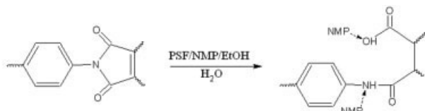
Scheme 3 Imide cleavage that leads to formation of amic acid and then complexation with NMP.
